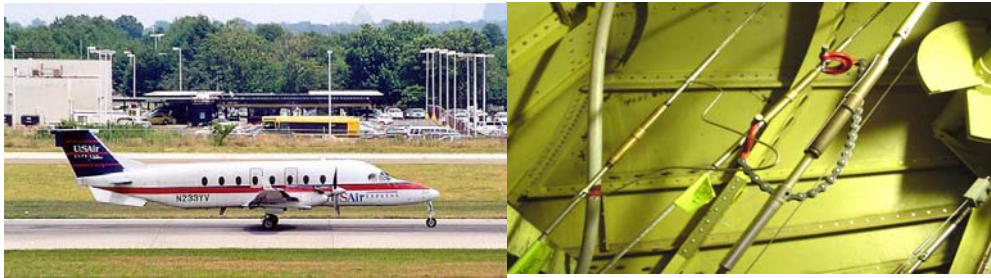
Figure 4: The Beech 1900 involved in the accident. Right, the cable adjustment turnbuckles on the elevator control cables.
